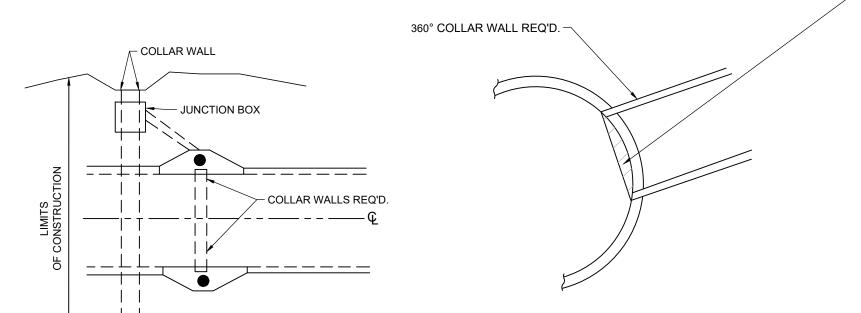
PIPE SHALL BE OF SUFFICIENT LENGTH FOR OUTSIDE DIAMETER TO REACH INTERIOR WALLS OF BOTH CATCH BASINS. UPON INSTALLATION, EXCESS PIPE SHALL BE REMOVED FLUSH TO INTERIOR WALL OF CATCH BASIN.
