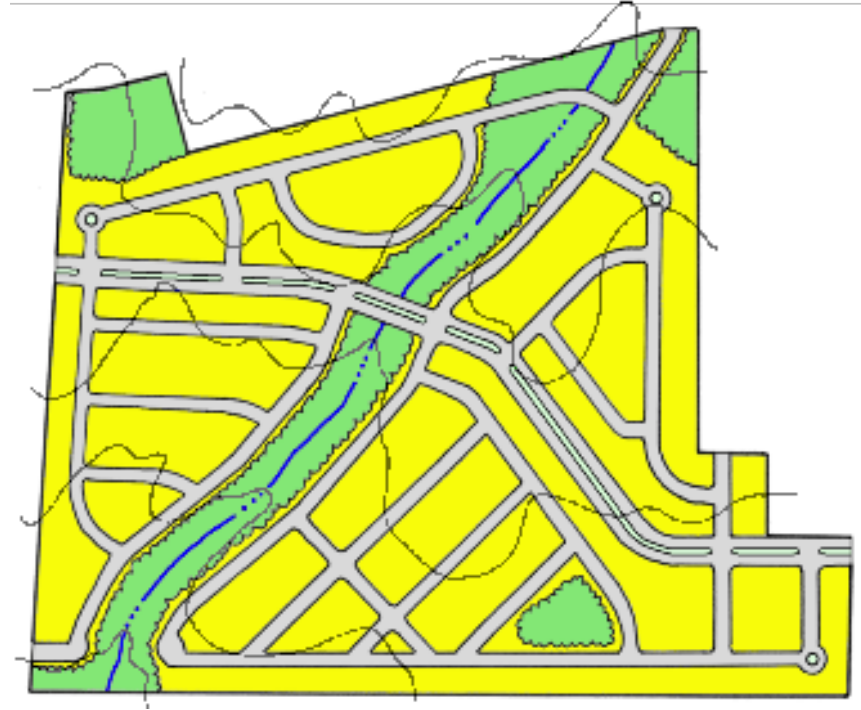
2.3.2-11 A Subdivision Design for Flat Terrain Uses a Fluid Grid Layout that is Interrupted by the Stream Corridor
