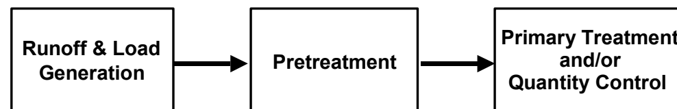
Figure 4.1.6-1 Generalized Stormwater Treatment Train
